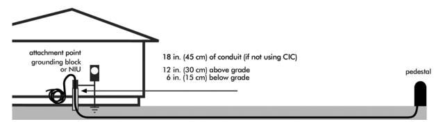
the earth. Place the conduit over the cable and run it down to the trench. Secure the conduit to the wall with Uclamps so that 6 in (15 cm) of cable is below grade and 12 in (30 cm) is above grade. Seal the end of the conduit with either a waterproof expanding foam or with a duct cap.
