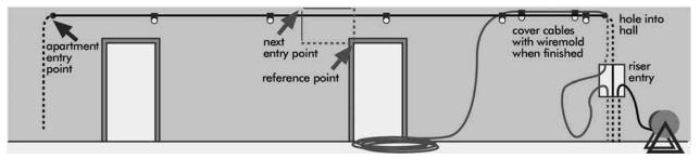
Use a stud finder to make sure you are drilling into a wall cavity. If possible, fish the cable down to the outlet location. Review Section 9 for details.
