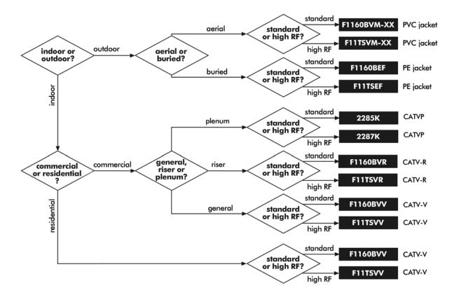
The XX in the part number should be filled with the code for the anti-corrosion agent you'd prefer as follows: **BW** for CommScope's dry BrightWire<sup>®</sup>, or **APD**<sup>\*</sup> for the more traditional APD flooding compound. All non-plenum high RF cables are Tri-Shielded (foil/60% braid/foil); super-shield versions are available. Plenum cables are available only with super-shields.
