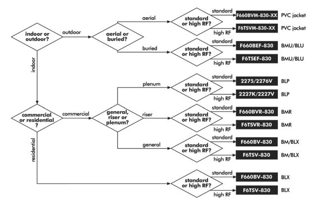
**BW** for CommScope's dry BrightWire<sup>®</sup>, or **APD**<sup>\*</sup> for the more traditional APD flooding compound. All non-plenum high RF cables are Tri-Shielded (foil/60% braid/foil); super-shield versions are available. Plenum cables are available only with super-shields. A 90% braid is available for 2276K.
