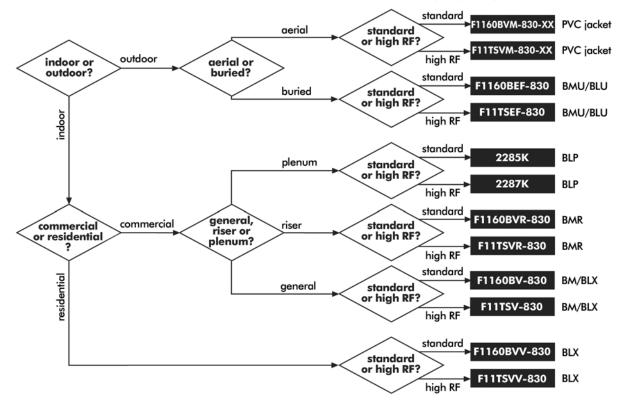
**BW** for CommScope's dry BrightWire<sup>®</sup>, or **APD**<sup>\*</sup> for the more traditional APD flooding compound. All non-plenum high RF cables are Tri-Shielded (foil/60% braid/foil); super-shield versions are available. Plenum cables are available only with super-shields.
